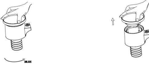
**Figure 11 Rain gauge installation and maintenance**
