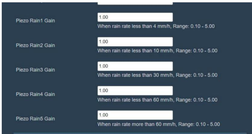
**Figure 10: Set five rain gain parameters**
