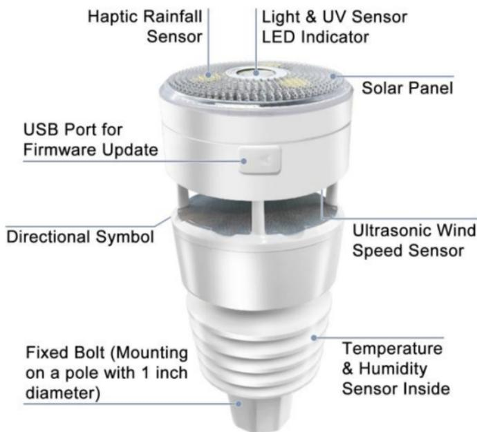
**Figure 2: Sensor package assembly components**
