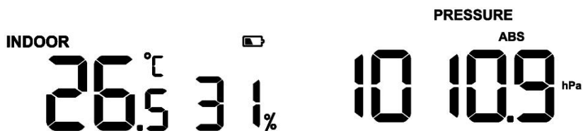
Figure 27: Indoor temperature, humidity, and pressure
